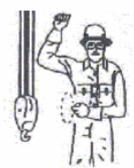
Travel: (one track crawler cranes) Lock the track on the side indicated by the raised fist, and travel opposite track in direction indicated by circular motion of other fist rotated vertically in front of body.
